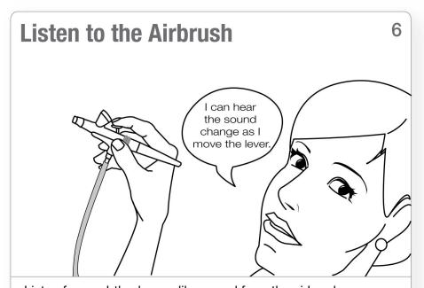
Listen for a subtle shower-like sound from the airbrush, as you gradually pull the lever back. You can hear when you are spraying lightly and when you are spraying too little or too much.
