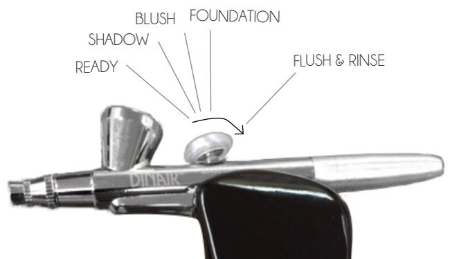
The Lever in the "Ready" position, Makeup off. You will feel a continuous air flow when the compressor is on. "Flush & Rinse" position is used to spray out makeup or cleaner quicker.
